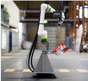
RAMLAB collaborative robot system combines 3D shape scanning and automated weld path generation for intelligent welding and printing automation
